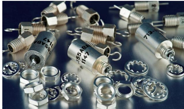
**Hermetic Filters:** Instec Hermetic filters utilize glass seals to achieve hermeticity and are ideal for applications where rugged, sealed filters are required. Internal designs consist of combinations of capacitors and inductors (ferrite beads or wire-wound inductors) in ¼-28 or 5/16-24 threaded cases. Given their larger sizes, very high capacitances can be achieved and higher current ratings are possible. Filter performance can be tuned to match the application by choice of inductors.
